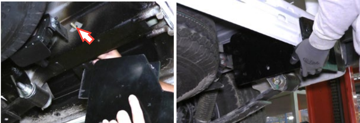
Position bumper frame mounts on the inboard side of chassis frame rails (RH shown)
