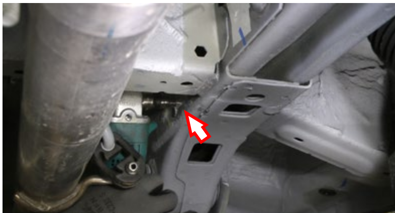
Enlarge hole in frame rail if necessary
