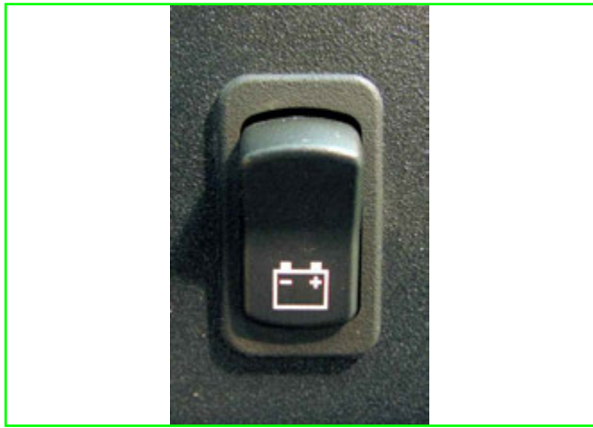
LOW VOLTAGE SWITCH
